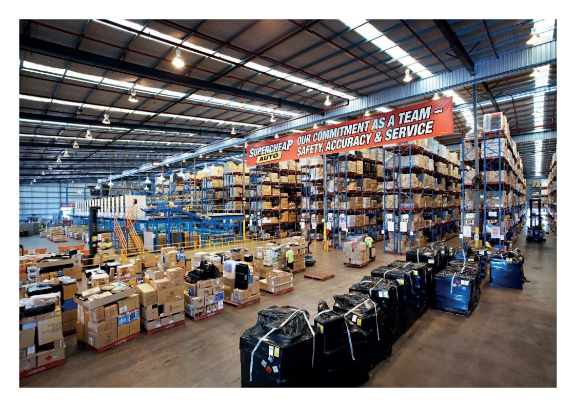
"Due to the rapid increase in volumes and the complexities of orders, Dexion introduced more sophisticated solutions and moved from paper based to RF picking as well as automating the movement of orders via conveyor systems to pick modules."
