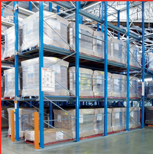
Each pallet sits on its own rails, so pallets no longer need to be stacked on top of each other.
