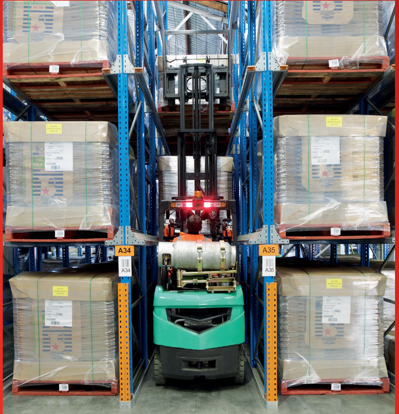
Handling equipment can drive right into the centre of the block between any upright on the front face to pick up pallets. Safety plays an important part in both initial design and installation allowing forklift operators to safely enter the structure.
