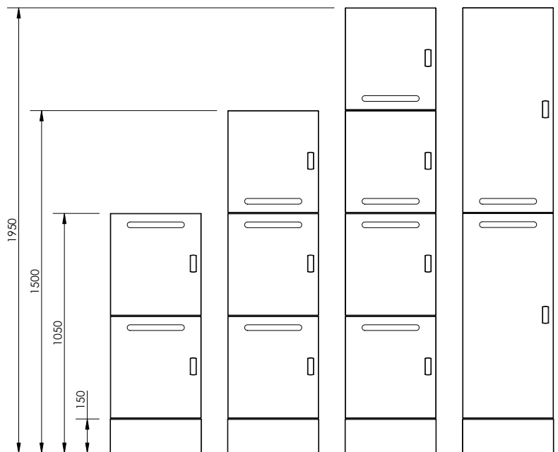
Kick-plate height is 150mm and add 16mm to heights when using a finishing top.
